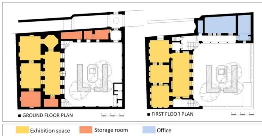
Fig. 10: a proposal for changing the Kian house into an art gallery or a small museum
